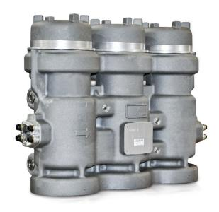
The QuickTrip trip block assembly is designed for use in steam, gas, and hydro turbine shutdown systems for quick and reliable dumping of the turbine's trip oil header. This integrated trip block assembly is intended for use on mechanical-drive or generator-drive steam turbines that use low pressure (5–25 bar / 73–363 psi) hydraulic trip oil headers.
