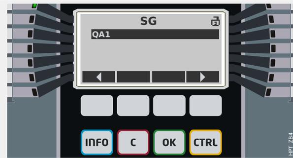
The Softkey “SG” takes you to a screen that lists all connected switchgear devices.
